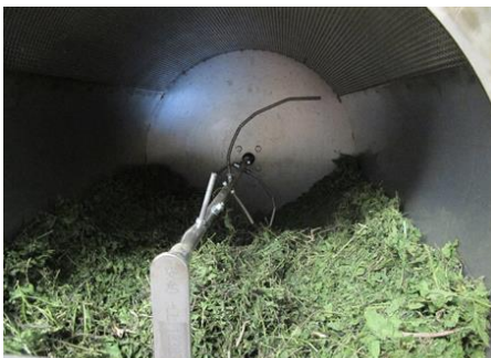
Figure 19. Dryer's interior with dried herbs.
