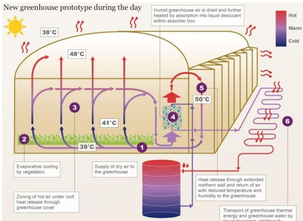
Thermochemical solutions allow to uptake a huge amount of heat during the hot period of the day by using the phase change between water vapor and water. Evaporative cooling of the plants is combined with the absorption process, which allows air dehumidification in the greenhouse atmosphere and heat transport from the air to a solution
