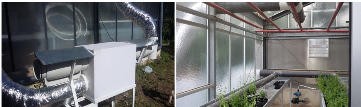
Fig. 9-10, Test stand at the experimental greenhouse in Tunis with experiments on improved heat dissipation to the outside and use of the absorption system.
