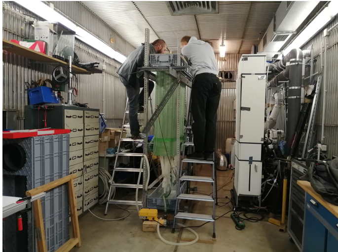
Workshop activities, optimising TCF distribution in the absorber using high flow velocities
