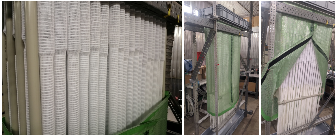
Fig. 42-44 New developed surface area for improved air distribution in botom-up direction, Absorbers integrating low cost components (pre-fabbed materials, plastic foil...)
