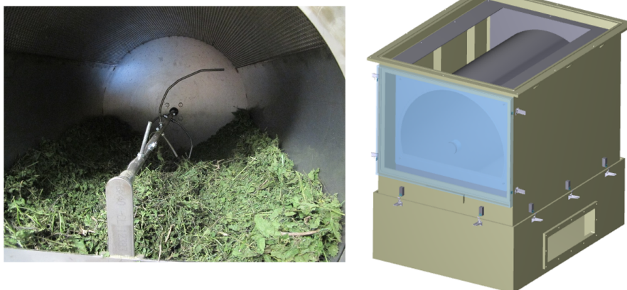
Figure 7: herbs inside the drying box of TheGreefa with the mechanism to turn the herbs (left) and its drawing (right)
