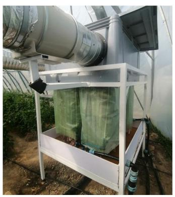
The hygroscopic property of the desiccant allows a higher dewpoint temperature in the daytime phase compared to a system only using water as a storage material. In this way, less cool (generated passively by nighttime temperature) is required for the process and cool is replaced by heat, as more heat is required during the regeneration phase, in order to regain the initial desiccant concentration for the next daytime phase.
