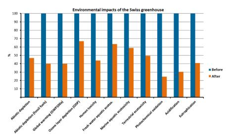
The results obtained in the LCA have shown that the use of the new TheGreefa technology in greenhouses contributes to visible lowering the environmental impacts of the greenhouse operations. The heating, and cooling humidity control are very energy intensive processes in the greenhouse operation.
