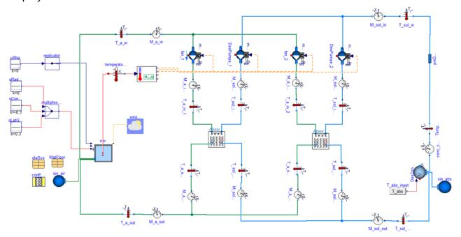
A three-stage control strategy (a small absorber on, a big absorber on and two absorbers on) is used to manage the system working conditions. Additionally, laboratory experiments are conducted to define the heat and mass transfer coefficient for model validation and calibration.
