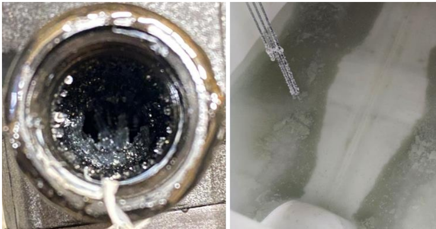
Figure 1. Membrane pump with crystal formation (left). Crystal formation in the concentrated solution tank (right).
