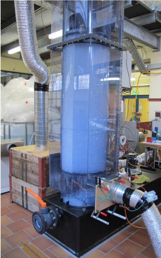
Figure 9. Transparent absorber at ZHAW-lab (left) and the absorber installed in the Swiss demonstrator (right).
