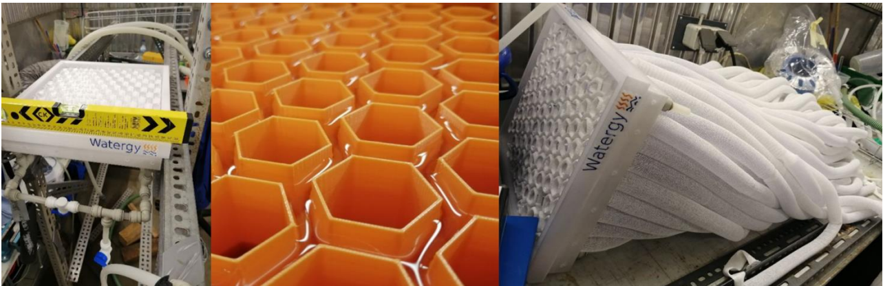
Figure 30. The absorber design with 3D printed hexagonal internal structure.
